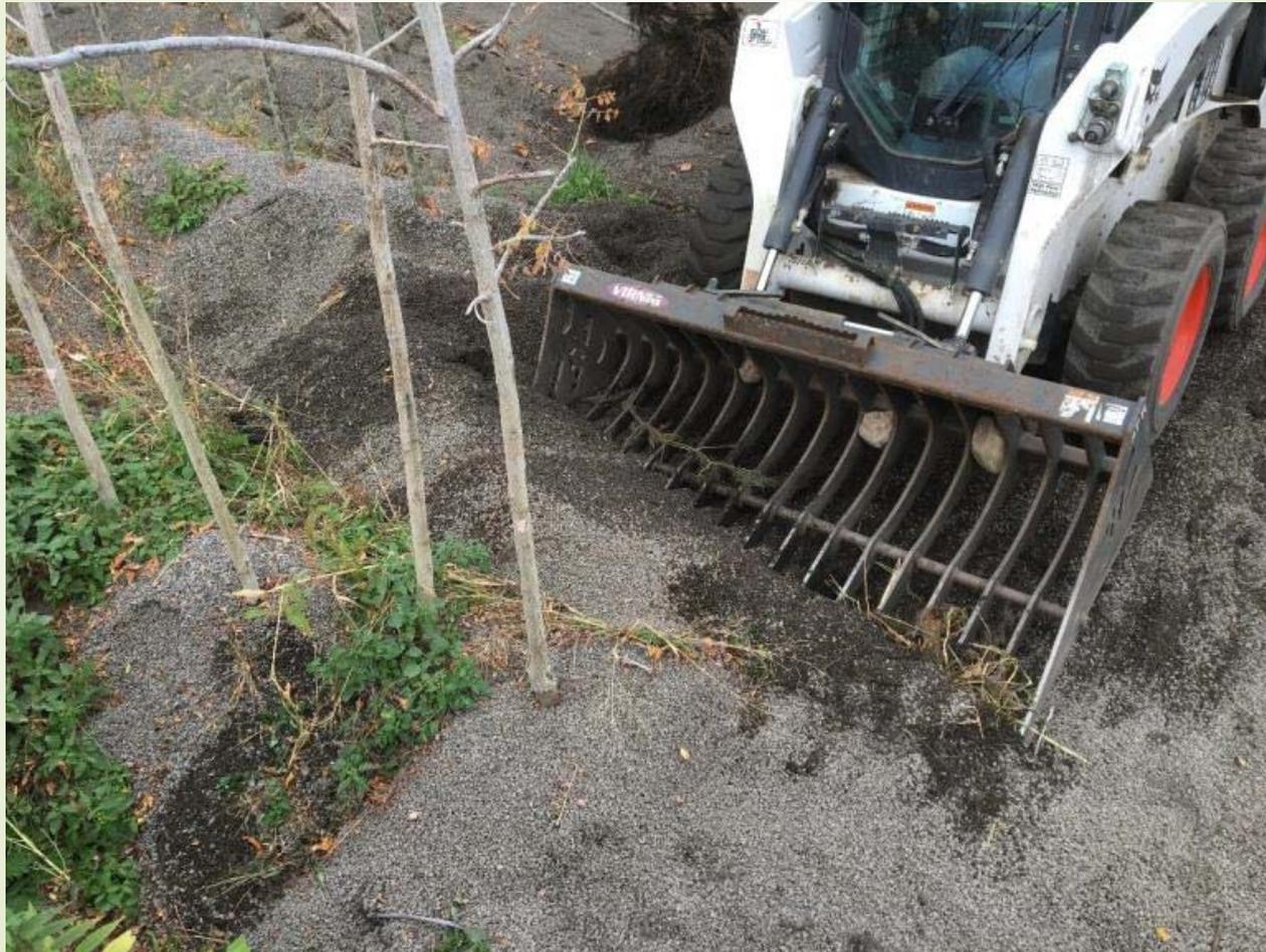
Front end loaders with a variety of buckets, forks or rakes is the fastest, least labor-intensive and best way of harvesting gravel bed trees with the maximum amount of roots retained. As you scoop up the gravel and tree roots, the gravel easily separates from the roots with a couple of shakes.
